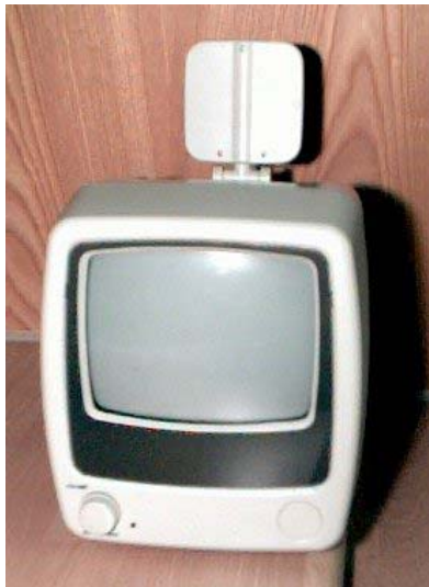
B/W monitor with integrated 2.4 GHz video receiver and white patch antenna on top. I use this monitor in the field next to the telescope for focusing etc.
