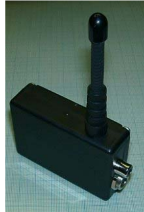
Video transmitter top view (connectors right are a RCA video input and power supply jack)
