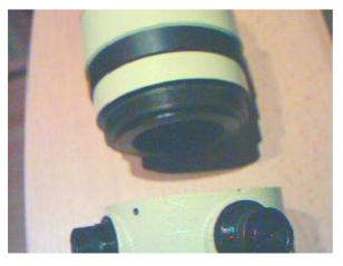
5) Now you can unscrew the top section from the bottom section. Please mark the spot, where the thread starts for easier reassembly of the eyepiece (to find the small indentation for the grub screws).
