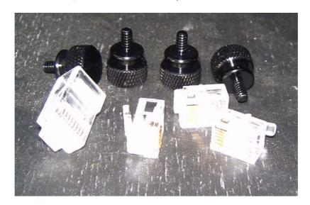
I shortened the threads of the thumbscrews and glued them into the blank connectors.
