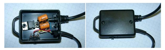
That's all. Finally a picture of the whole device with a cable supplying the  $+10 \dots 20V$  input voltage and the Western plug with the output voltage for the DECT-terminal.
