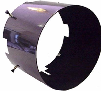
When starting to use the N11GPS for imaging using my Casio digital camera in afocal configuration, I soon learned how critical proper focusing is. So I thought about building a classical Hartmann mask by cutting 2 or 3 holes in a cardboard mask. However I did not like the large dimension of such a mask which is only needed a few minutes during a session and the rest of the time only taking space ...
