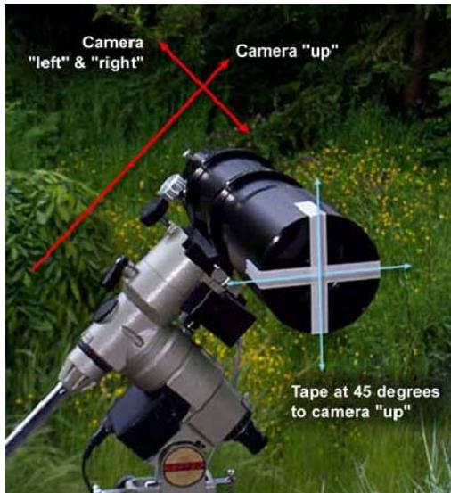
Browsing the internet for an alternative solution I found the book "The New CCD Astronomy" of Ron Wodaski. In chapter 2 "Practical focusing" he explains in section 4 the different options of "Aids to Focusing". I especially liked the idea of adding an artificial spider in front of the OTA to create diffraction spikes, which can be used for proper focusing. For further details please see this section of Ron Wodaski's book online at <http://www291.pair.com/rwodaski/ebook/c2d.pdf>
