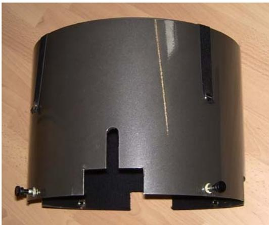
By the way the location of the 4 holes is easy to determine: you hold the stripes diagonal over the opening of the Dew-Shield and stretch them symmetrically down along the sides of the Dew-Shield while keeping under moderate tension. Here you now mark the points to drill the holes.
