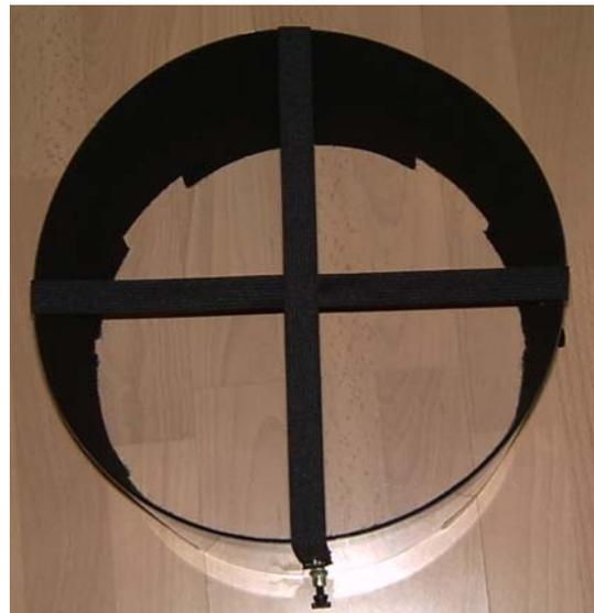
Finally here are 2 pictures of the stripes while not in use. They are wrapped around the Dew-Shield and thus securely stored. As you can see we met our target of having an easy to use focusing aid which takes virtually no additional space when not in use.
