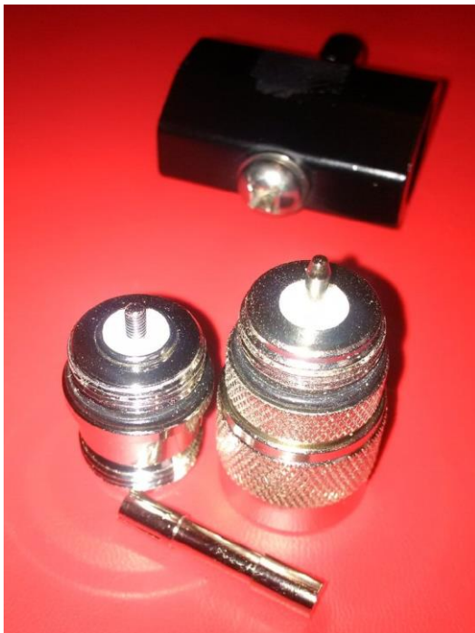
The N-Plug has a threaded center pin
