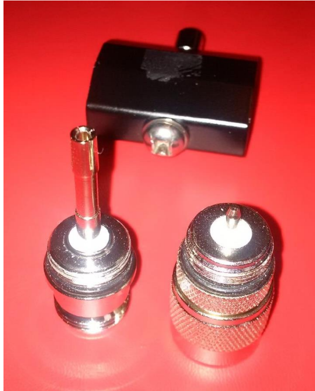
The inner conductor is screwed to the N-Plug and clamped to the N-Jack
