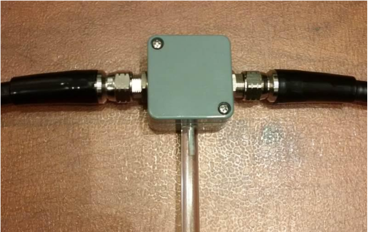
This isolating plastic box provides the mechanical connections of the coaxial cables and the Plexiglas rod...
