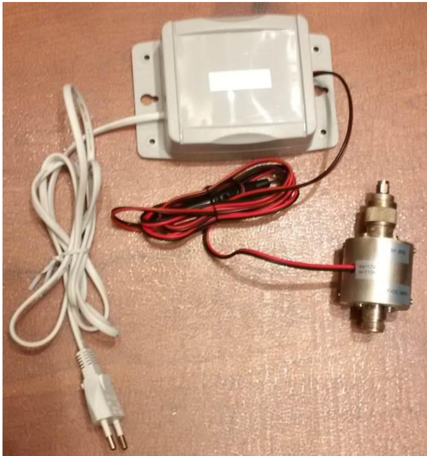
This is the 12V power supply and the Bias-T. The power supply is using a 7812V linear voltage regulator IC to avoid any interference.
