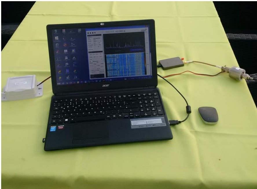
The laptop is running SDR# in combination with the Airspy HF+ SDR
