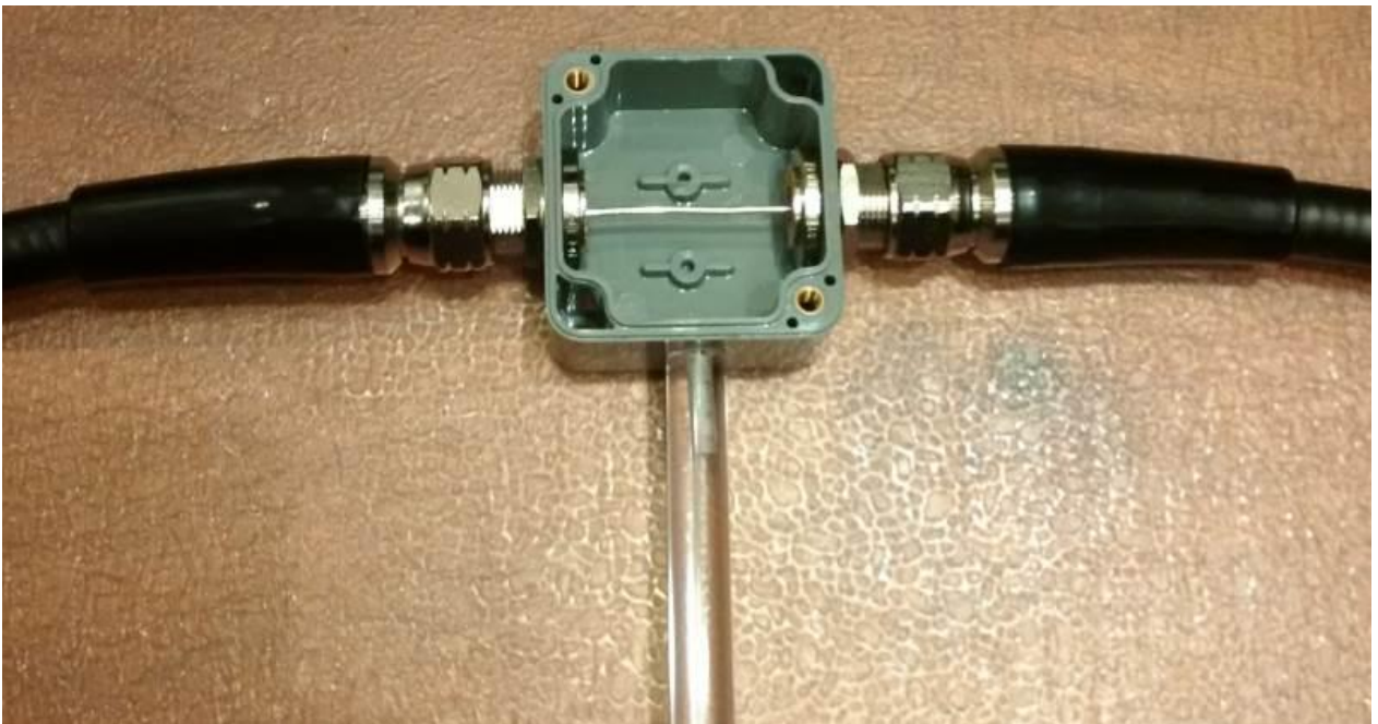
... as well as the connection of the inner conductors of the coaxial cables.
