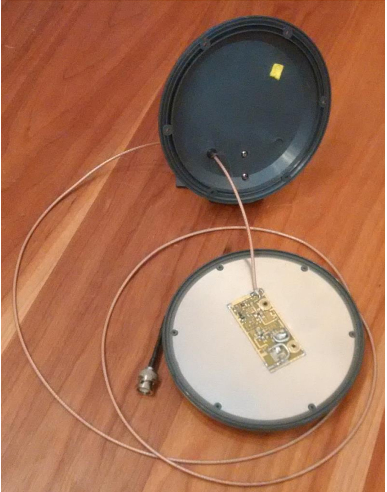
Now only the shielding is missing before closing the plastic encasing
