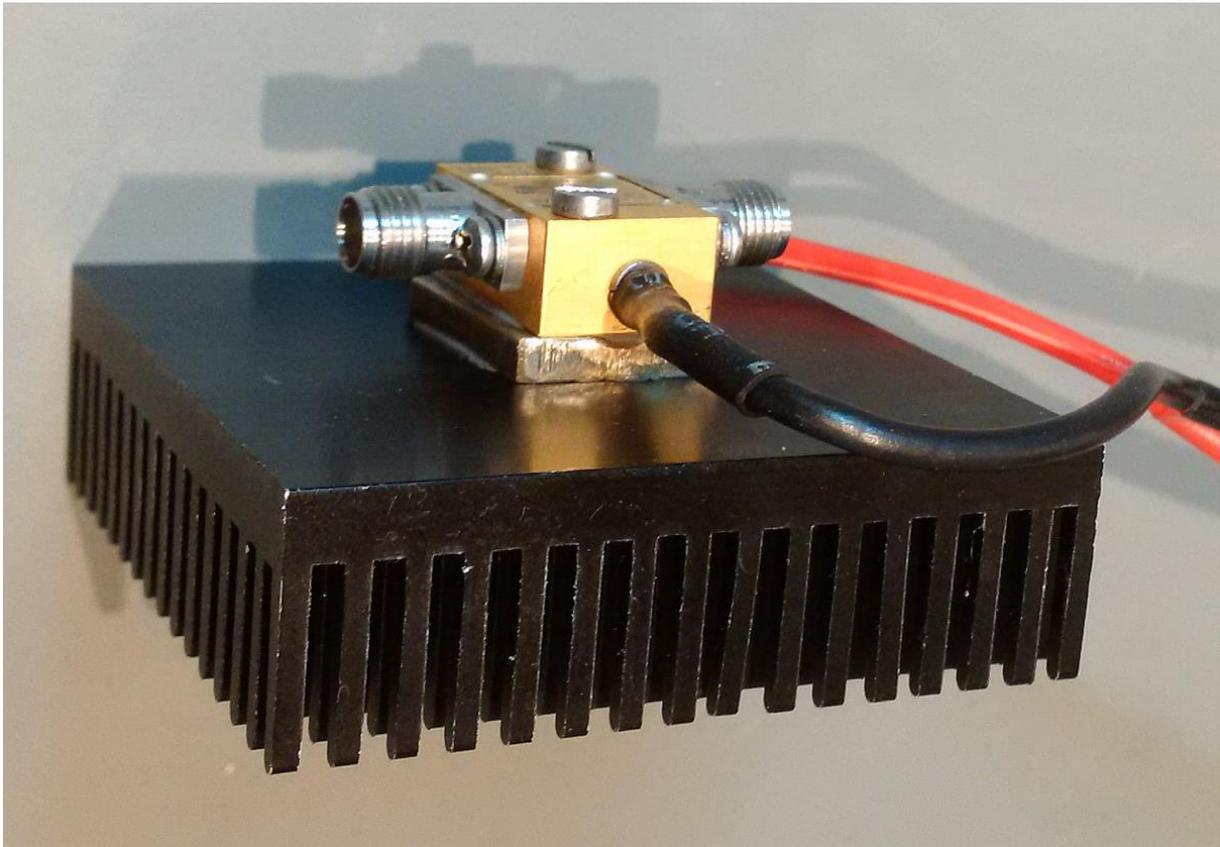
First, I measured gain and noise figure in the frequency range 50MHz to 3500 MHz:
