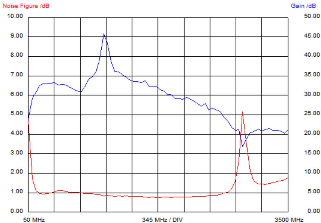
The graph for gain and noise figure are almost the same with gain being about 1dB higher at frequencies below 2 GHz and the noise figure being about 0.1dB better. Here are the respective values:
