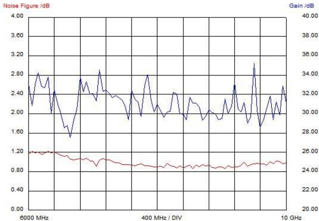
As can be seen both diagrams are virtually identical. The gain is about 32dB in this wide frequency range. The noise figure is 1.2dB at the lower end and about 0.9dB in the center. Thus, the device has higher gain and lower noise figure than the specified values.
