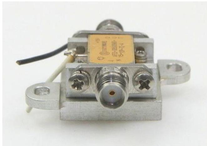
I have not yet mounted the amplifier on a heatsink but will do so as I measured a current consumption of 100mA at a supply voltage of 15V. Also, at 12V the supply current is almost 100mA. As the amplifier dissipates quite some heat it is certainly better to keep it cool using a heatsink as low noise figure and high temperature do not get along well.
