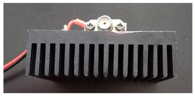
Next, I measured gain and noise figure versus frequency. The first measurement was done at the nominal supply voltage of 20V and a corresponding supply current of 110mA.
