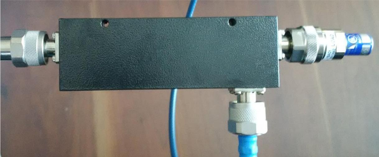
The isolation including the 30dB coupling factor was measured to be 80.5dB at 1.3 GHz and 56.3dB at 2.4 GHz respectively.
