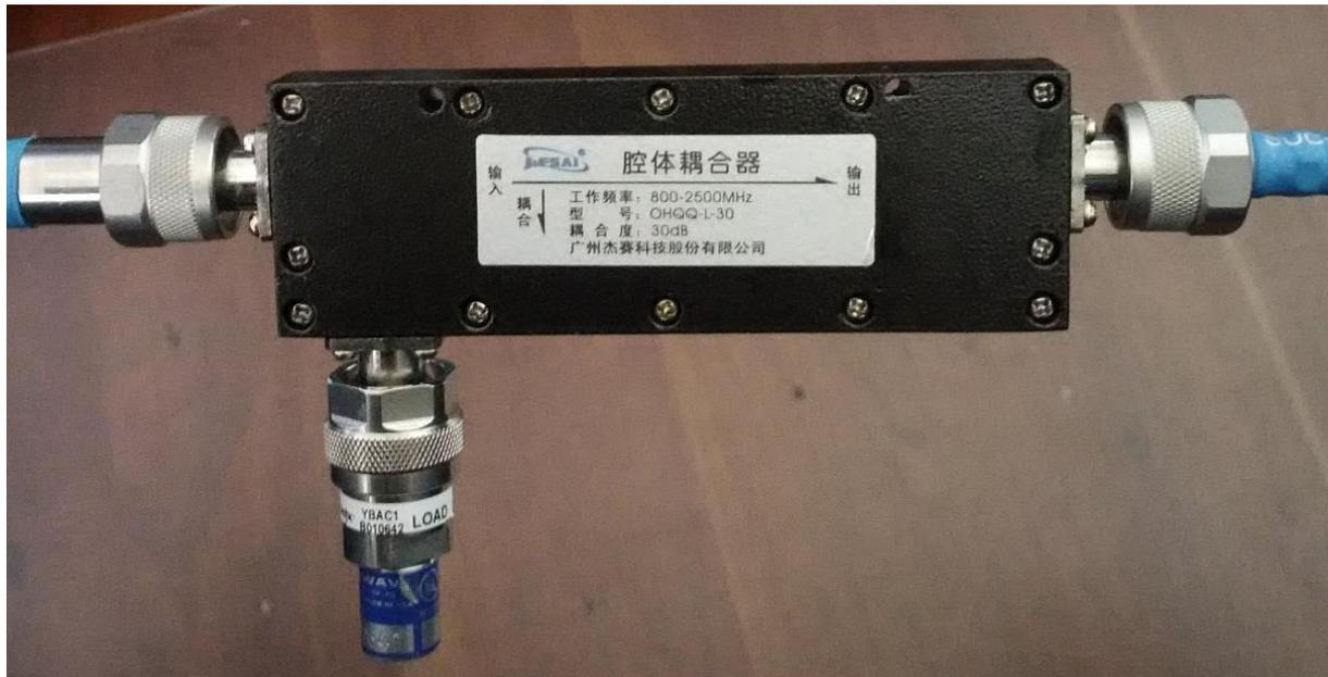
As can be seen in the next graph the insertion loss at 1.3GHz was measured as 0.012dB and at 2.4 GHz as 0.034dB. This is well in the spec of better than 0.05dB.
