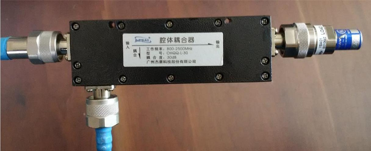
As can be seen in the next graph the coupling factor at 1.3 GHz was measured as 29.6dB and at 2.4 GHz as 29.8dB. This is amazing close to the specified value of 30dB for such a low-cost device.
