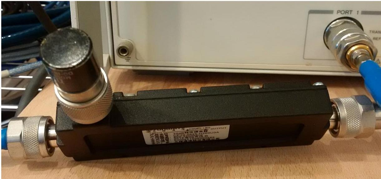
As can be seen in the next graph the insertion loss at 1.3GHz was measured as 0.08dB and at 2.4 GHz as 0.12dB. This is slightly higher than the spec of better than 0.05dB.
