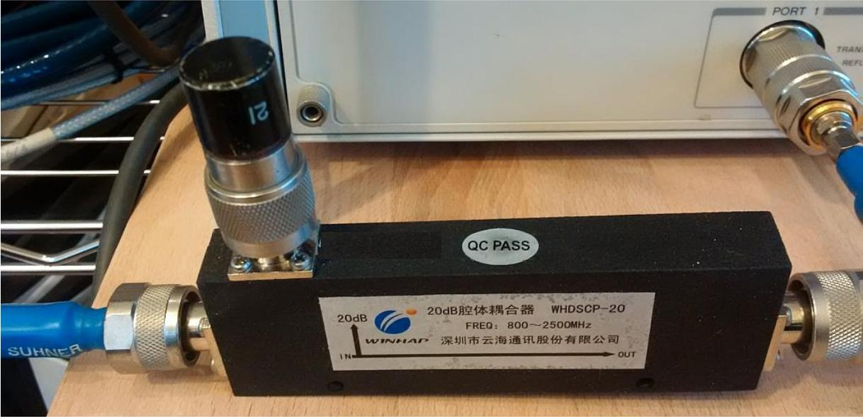
As can be seen in the next graph the insertion loss at 1.3GHz was measured as 0.087dB and at 2.4 GHz as 0.156dB. These values are slightly worse than the specified values of better than 0.05dB.
