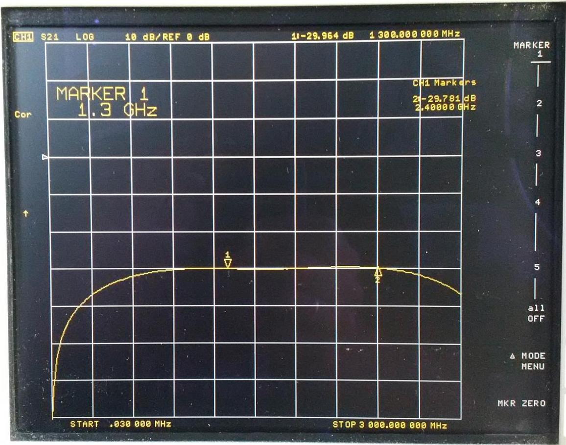
Next, I measured the isolation S23 from the output port to the measurement port. The input was again terminated with a high quality 50 Ohm load.
