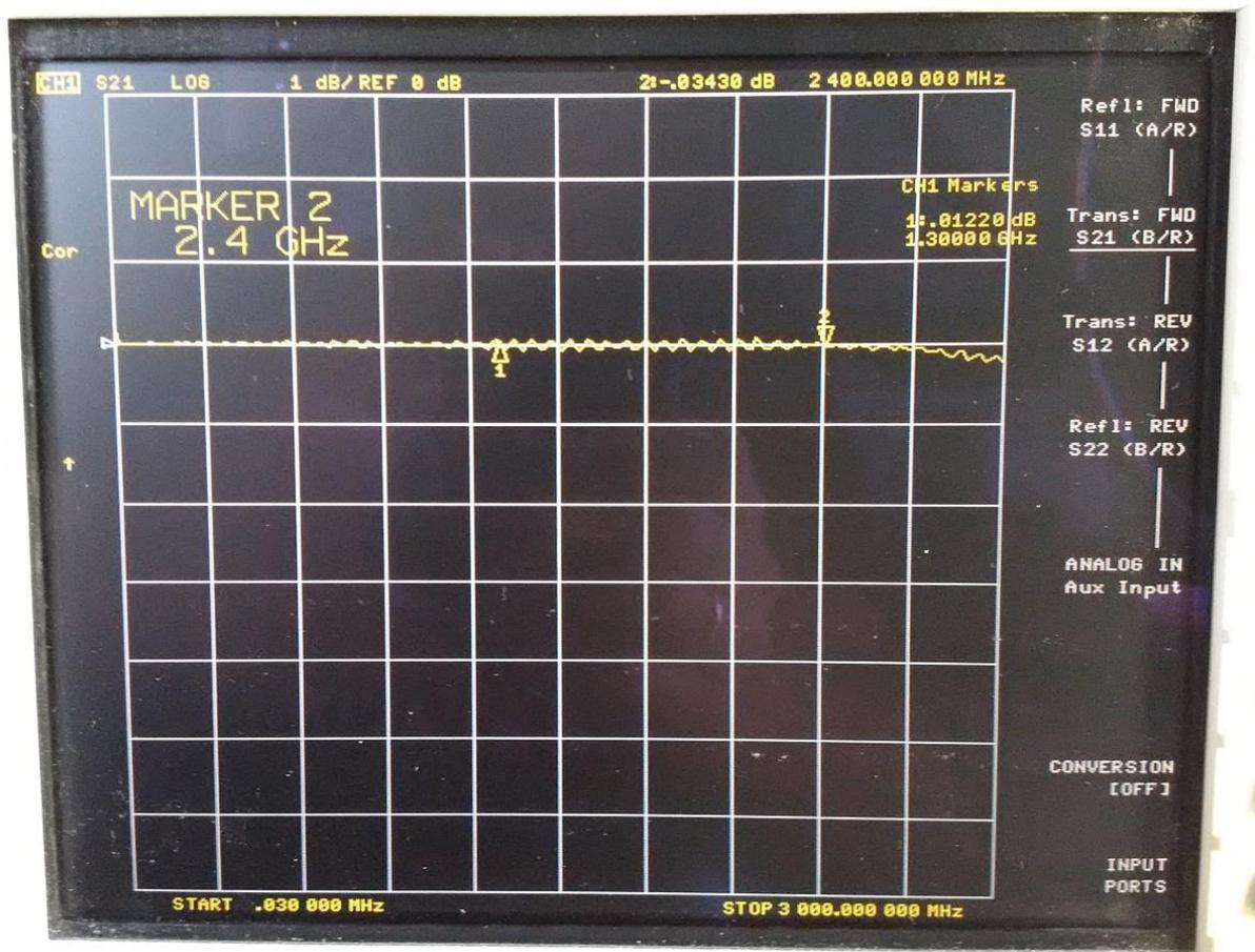
I have not tested the maximum power but the very low insertion loss indicates that there should be no problem. The insertion loss of 0.034dB means that using an input power of 200W less than 2W are dissipated in the coupler.
