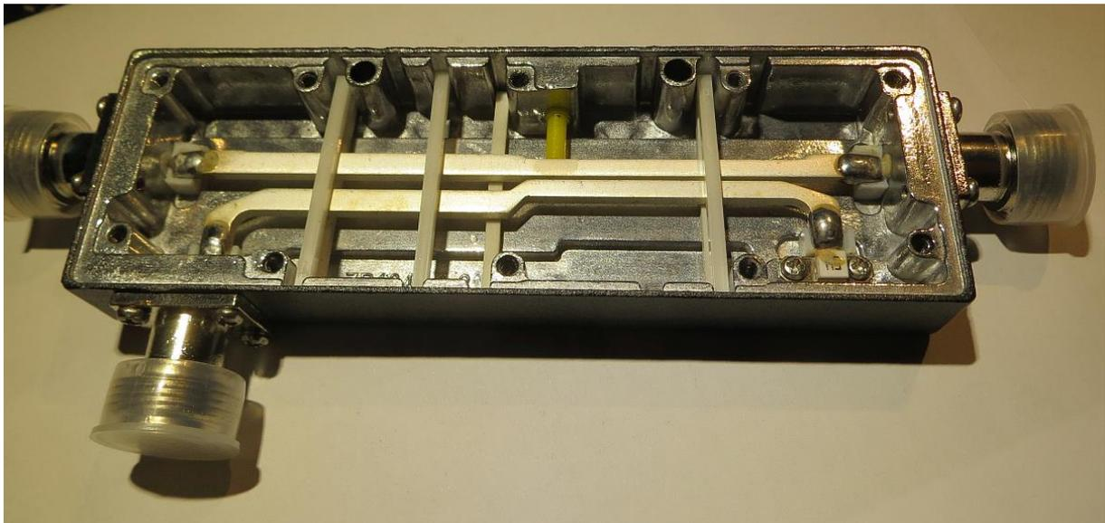
Please note that yellow plastic screw which can be moved from outside. This screw is pushing against the upper transmission line (bar) and thus the distance to the second line can be adjusted. Thus the coupling factor can be tuned in production. After alignment a sticker like QC or similar is glued over the screw to hide / protect it.
