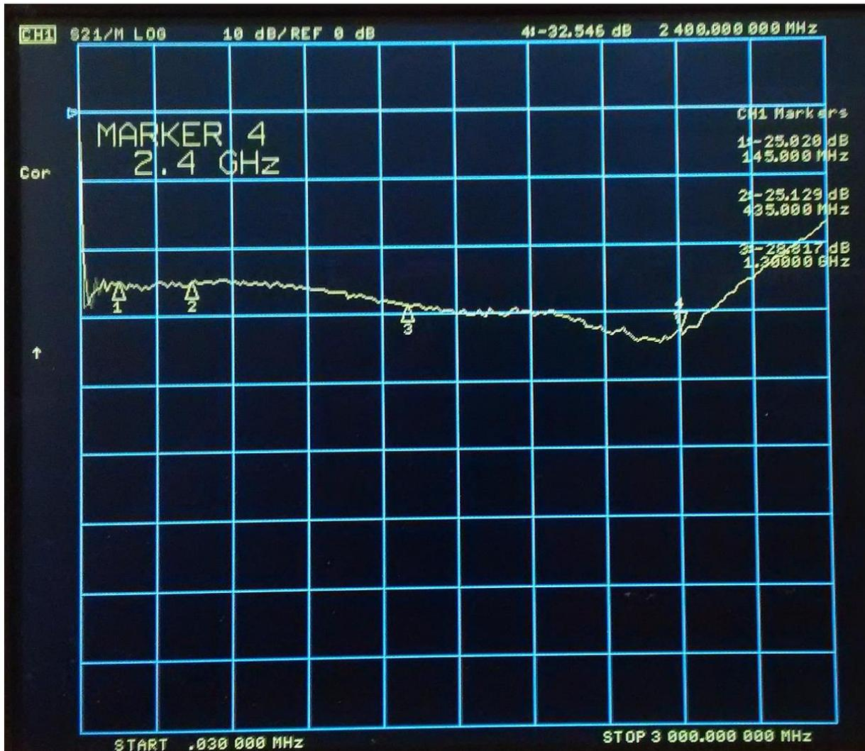
The directivity was measured to be 28.8dB at 1.3GHz and 32.5dB at 2.4GHz respectively. This is significantly better than the specified value of >20dB. This coupler works especially well at the 13cm ham radio band.
