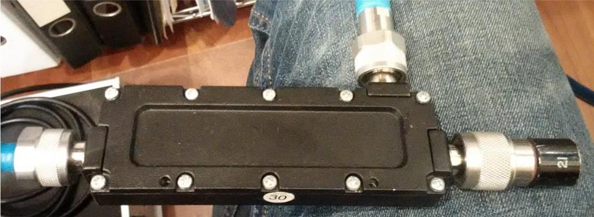
The isolation including the 30dB coupling factor was measured to be 58.6dB at 1.3 GHz and 63.9dB at 2.4 GHz respectively.
