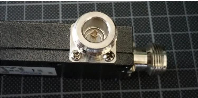
First, I measured the insertion loss S21 of the coupler from 30kHz to 3 GHz with the measurement port terminated with a high quality 50 Ohm load:
