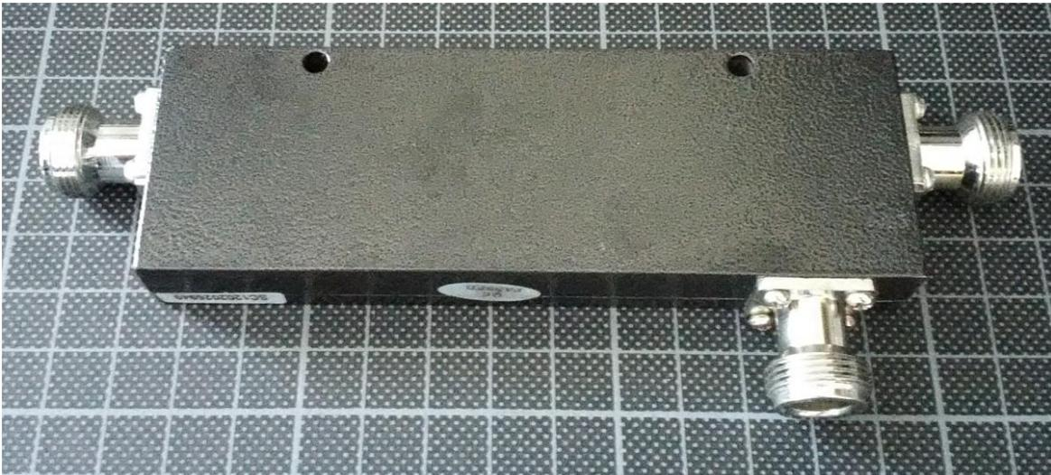
The N-connectors are not really high quality but should be ok if the unit is used in a permanent setup as I am planning for. The outer thread is reasonably precise so that the N-Connectors can be easily screwed on.
