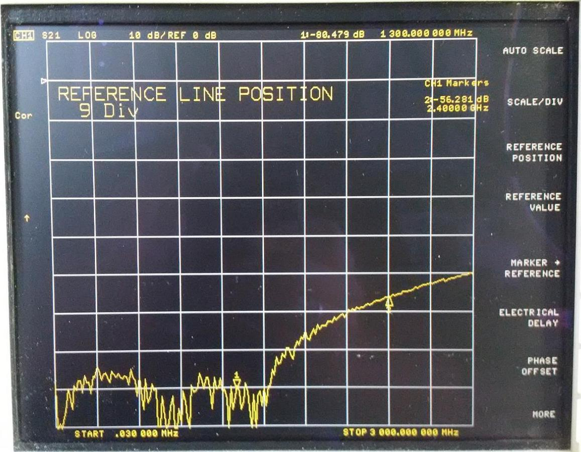
Finally, I measured the directivity, which is the ratio S31 to S32.
