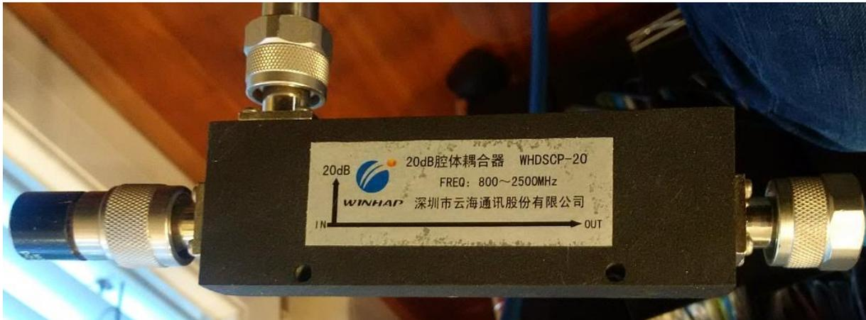
As can be seen on the next plot the isolation including the 20dB coupling factor was measured to be only 45dB at 1.3 GHz but amazing high 70dB at 2.4 GHz. Exactly at 2.4 GHz this coupler shows a strong resonance with respect to its isolation.
