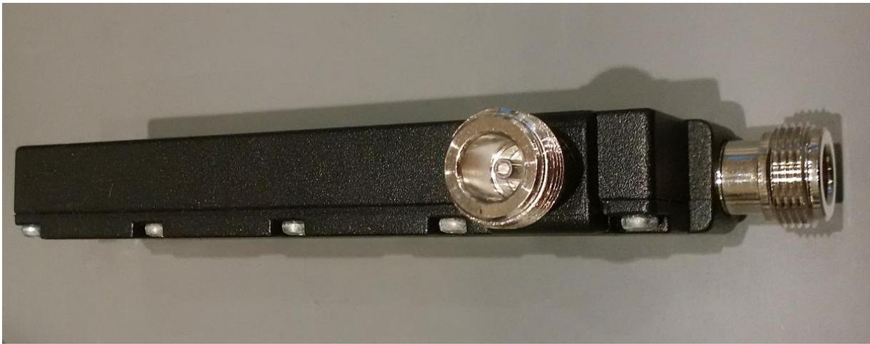
The N-connectors are not really high quality but should be ok if the unit is used in a permanent setup. The outer thread is reasonably precise so that the N-Connectors can be easily screwed on.
