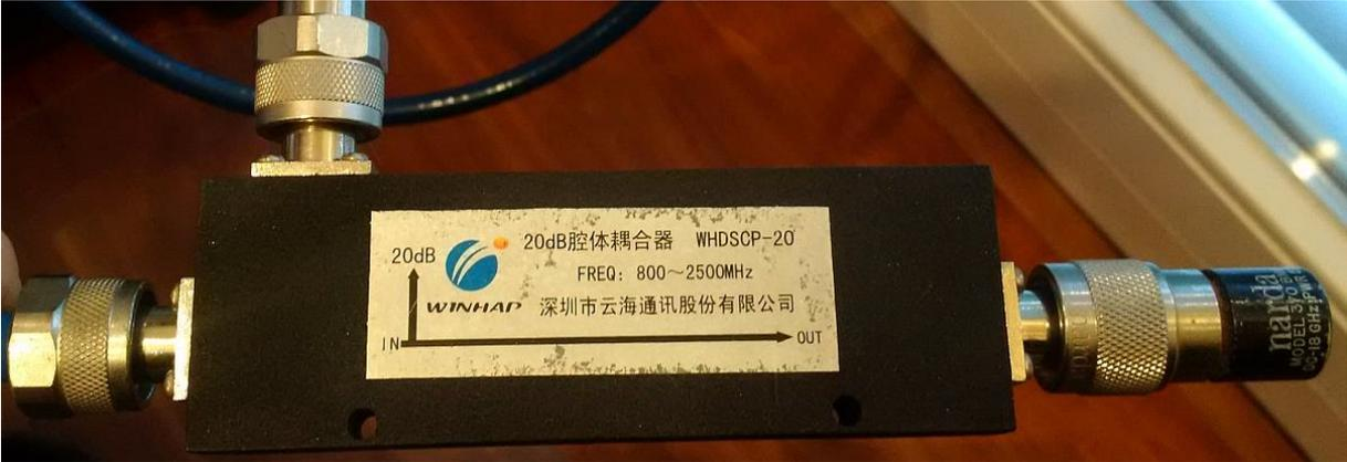
As can be seen in the next graph the coupling factor at 1.3 GHz was measured as 19.55dB and at 2.4 GHz as 19.75dB. This is amazing close to the specified value of 20dB for such a low-cost device.
