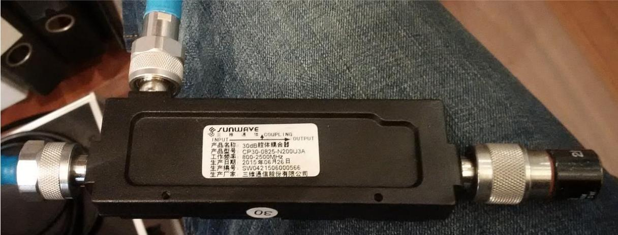
As can be seen in the next graph the coupling factor at 1.3 GHz was measured as 29.94dB and at 2.4 GHz as 30.19dB. This is amazing close to the specified value of 30dB for such a low-cost device.
