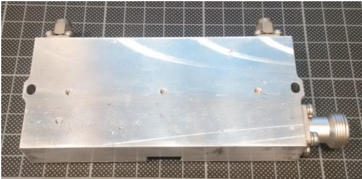
Bottom view of the branch-line coupler
