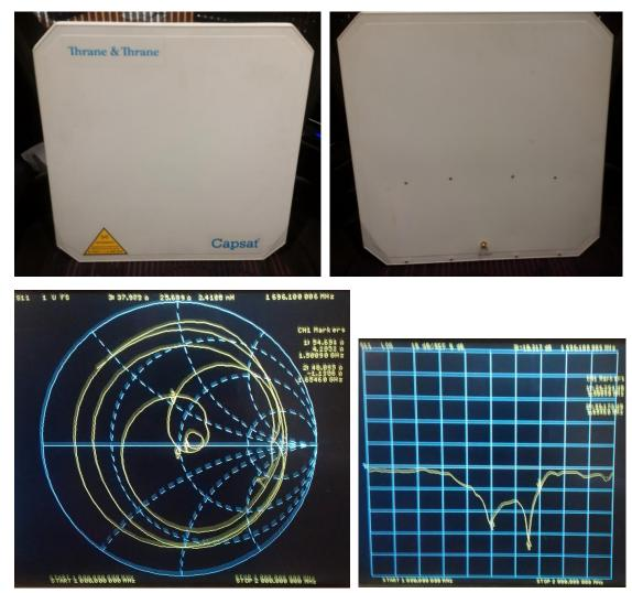
There are two resonances: one for RX with a return loss RL=24dB @1500MHz and another one for TX with a return loss RL=33dB @1650MHz.
