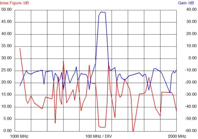
In the specified receive frequency range the gain is about 38dB and the noise figure better than 1.7dB. This is an excellent value as it includes the losses of the duplex filter.
