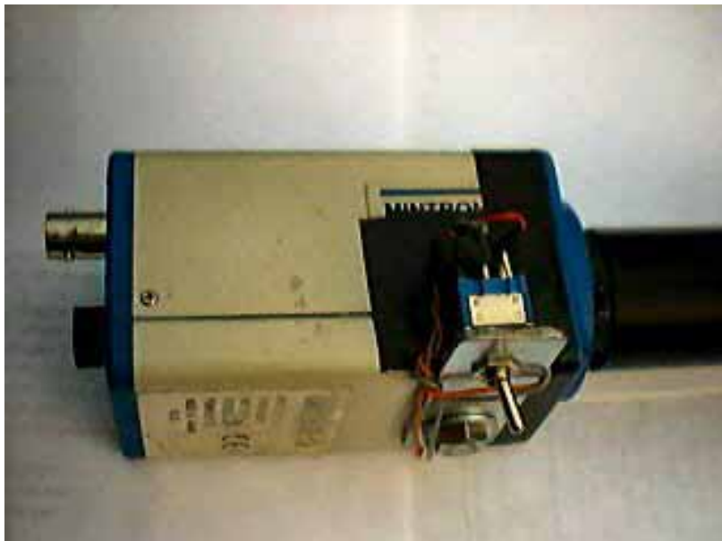
Image 1 Modified Mintron (the orange and grey wires are used for my light-on modification)
