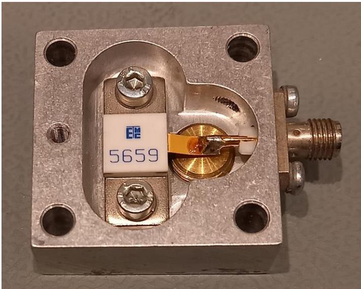
The 50 Ohm resistor is housed in a ceramic package made from BeO with a solid flange. It is screwed in the aluminum encasing to ensure a low thermal resistance. The input pin to the resistor is a rather wide terminal lug and the return loss can be tuned with a brass screw from the back of the encasing (changing the capacitive loading of the input).
