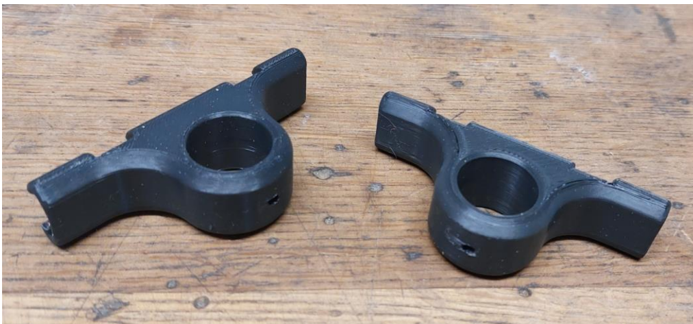
Picture 4-8: 3D printed element holders for radiating elements and reflectors/directors
