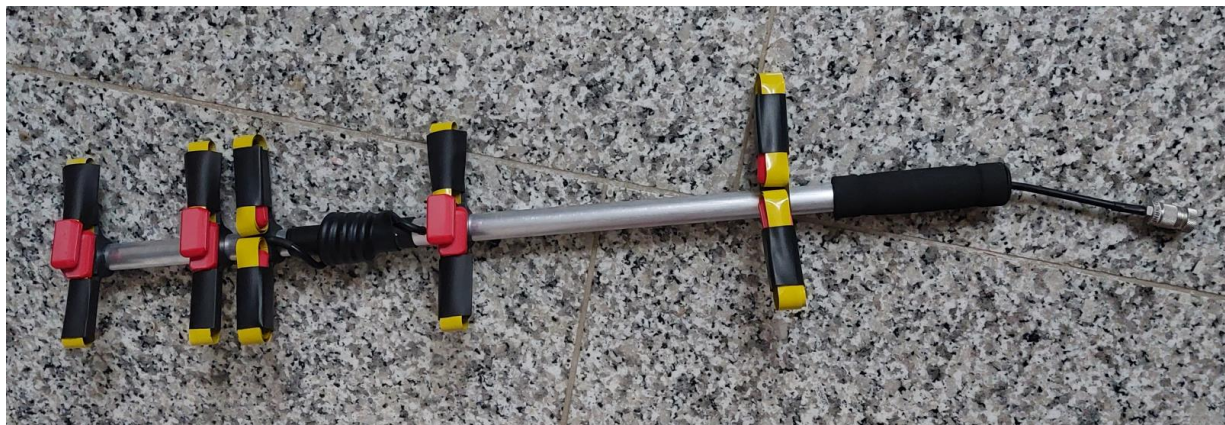
Picture 18: Antenna elements rolled up for transport and storage
