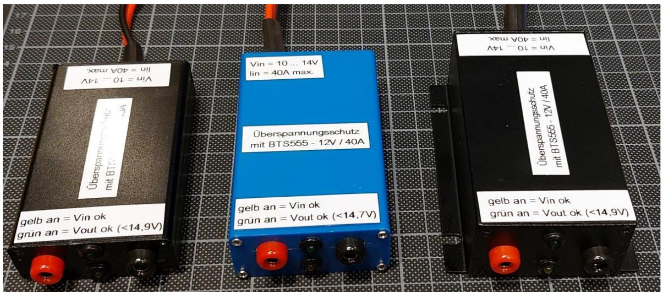
I can highly recommend to add an overvoltage protection to your main power supply in the shack. Often several expensive transceivers or other equipment are connected to one power supply which will result in significant damage in case the power supply fails
