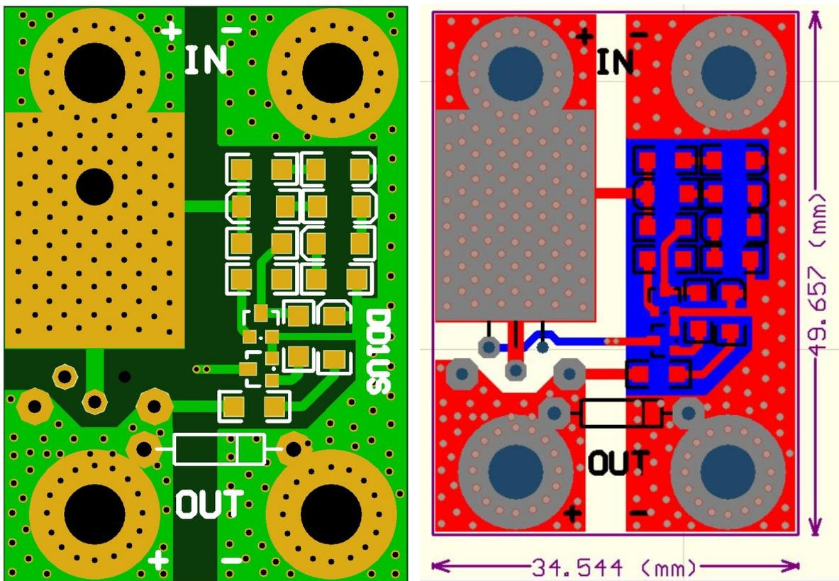
With the selection of the Zener diode voltage and one or two series diodes you can select the voltage, at which the unit will trigger the over voltage protection. In my case I am using a 12V Zener diode plus two series diodes resulting in a trigger voltage of 14.3V.
