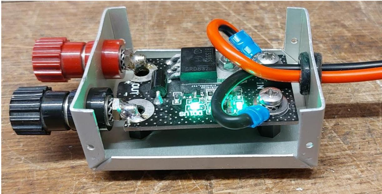
There are 2 LEDs on the board indicating the input and output voltages being present. In order to have them still visible after adding the lid on the encasing I integrated 2 acrylic rods routing the optical signals from the SMD LEDs on the PCB to the top of the lid. In the following pictures you see on the left both LEDs active as the unit is working nominally and on the right side only the input LED active as the output is shut off due to an overvoltage condition.
