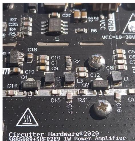
First, I measured the device first at 1300 MHz as I was considering to use it as a driver amplifier for my HPA in the 23cm ham radio band. With a supply voltage of 12V the current consumption was 386mA. Thus, the input power is 4.6 W.
