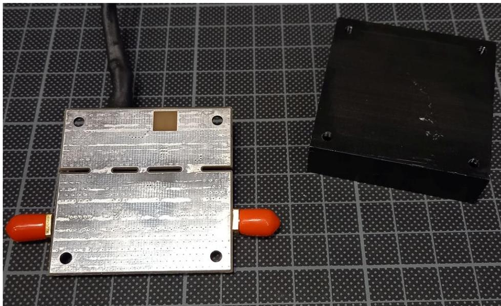
Therefore, I added 2 M2.5 screws close to the second MMIC and mounted the PCB on the heatsink with some thermal grease (Arctic 5).
