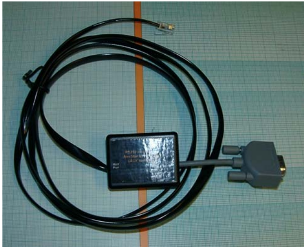
Completed Converter in encasing with cabling
