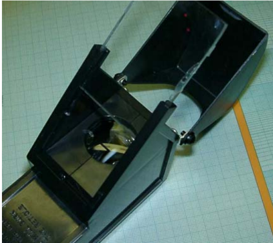
Fig.3: The projection window can be easily removed. It is glued in the plastic frame only by some silicone type of adhesive.
