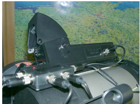
Fig.7: Telrad with closed dew shield from the rear. Please note that the dew shield alone (without additional heating) was not sufficient.
