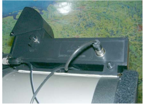
Fig.6: Telrad after modification mounted on N5. An additional socket was mounted which provides continuous DC power for the Telrad itself as well as pulse width controlled DC power for the heater only. Thus the Telrad and the heater can be powered independently
