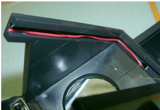
Fig.4: A thin wire (Konstantan) is laid around the window. This wire acts as the heater dissipating some power while the current is flowing through it. It has to be partly isolated (red isolation visible) to avoid short circuits. The ends are routed through a small existing opening inside the Telrad.
