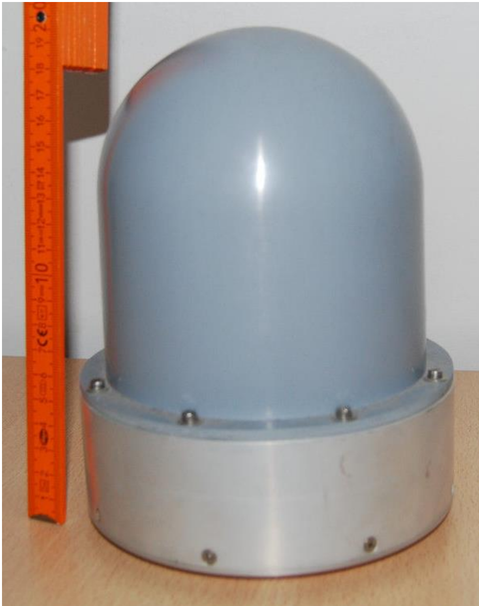
Complete antenna with fibre glass radome
