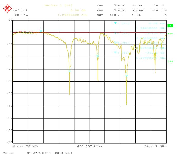
Please note that the measured depth of the notches is not precise due to the wide frequency span. Therefore, please find the measured insertion loss zoomed to the 2<sup>nd</sup>, 3<sup>rd</sup> and 4<sup>th</sup> harmonics in the next 3 diagrams. The scaling of the horizonal axis is 50MHz/div. and of the vertical axis it is 10dB/div.
