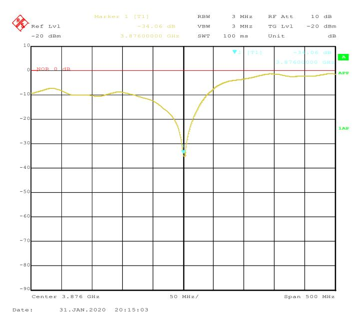
The measurement with the spectrum analyzer with integrated tracking generator shows an insertion loss at the 3<sup>rd</sup> harmonic at 3876 MHz of 34dB.
