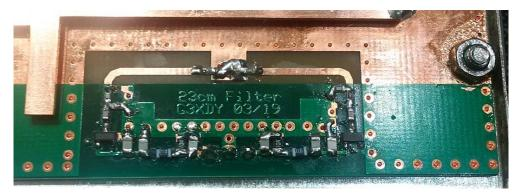
I am fortunate to have access to a VNA up to 3GHz and a spectrum analyzer with tracking generator up to 7 GHz. As John suggested I first tuned the transmission line for minimum insertion loss and maximum return loss using the VNA by bending the transmission line slightly towards the copper plated ground-plane. Also tuning the open stubs following his recommendations works perfectly well. Here are my final results:
