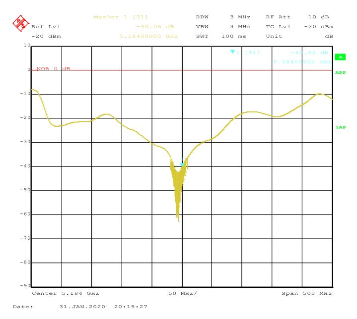
The measurement with the spectrum analyzer with integrated tracking generator shows an insertion loss at the 4<sup>th</sup> harmonic at 5184 MHz of 40dB.
