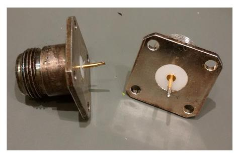
Here are some pictures of the finished unit housed as John proposed in a tin-plated cabinet with the dimensions 55x148x30mm. I decided to solder the silver- plated N-jacks to the box lid to ensure good grounding and improved mechanical stability.
