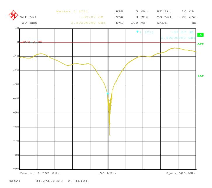
The measurement with the spectrum analyzer with integrated tracking generator shows an insertion loss at the 2<sup>nd</sup> harmonic at 2592 MHz of 37dB. The notch is very narrow and deep which is a result of the very high quality factor of the quarter wave stub for the 2<sup>nd</sup> harmonic at 2592 MHz
