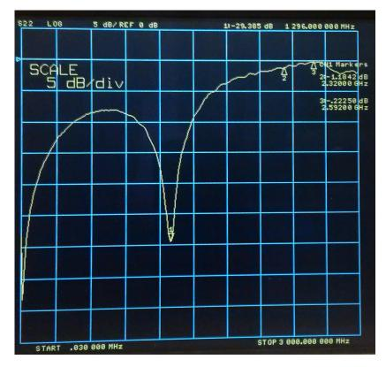
The output return loss at 1296 MHz is 29dB which corresponds to a VSWR of 1:1.07 or a reflection coefficient of 0.11%.
