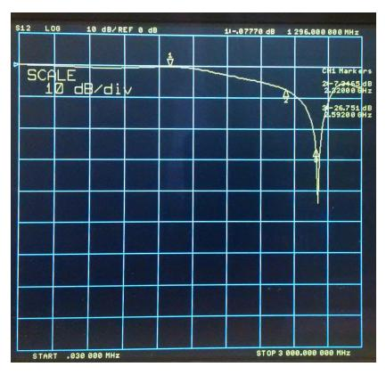
As to be expected the filter is symmetric, thus S12 is basically identical to S21.
