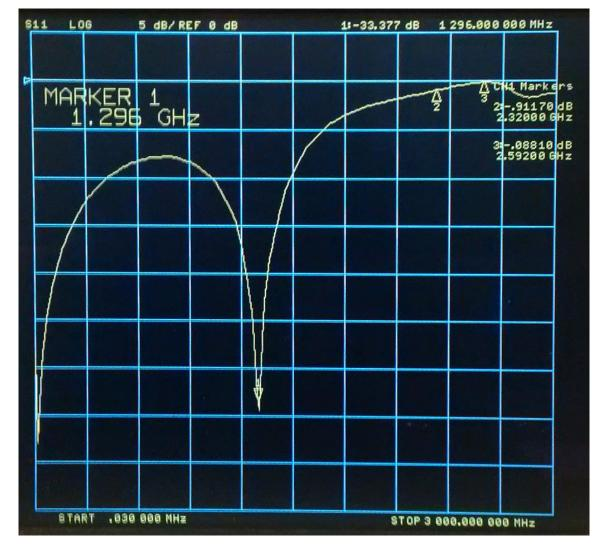
S11 input matching (hor. axis 300MHz/div, vert. axis 5dB/div):
