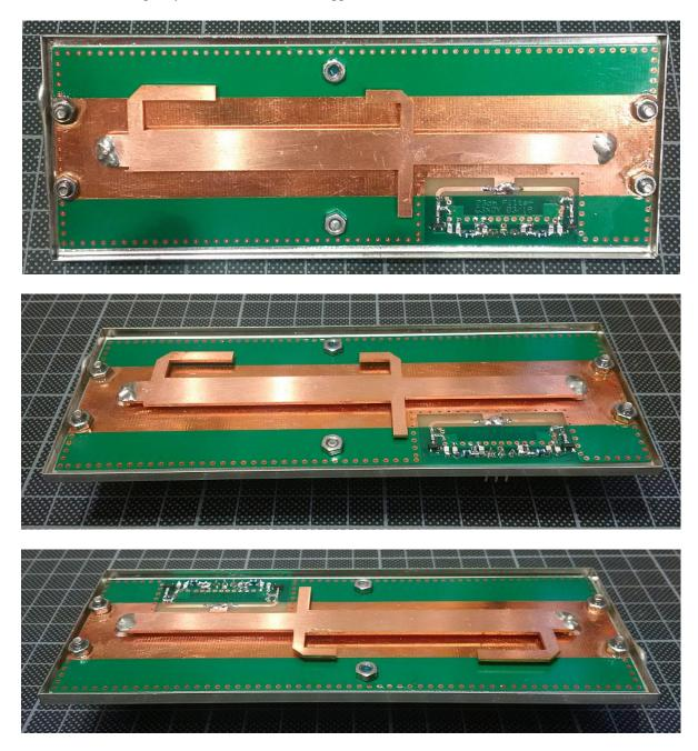
Here is a closer look at the reflectometer comprised of the directional coupler, 2 double diode detectors Infineon BAS70-04 and some passive components:
