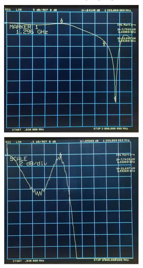
The insertion loss at 1296 MHz is approximately 0.05dB and thus amazing low. This is perfect especially for using the filter at high power levels. You can see also the function of the first notch at 2592 MHz: the 2<sup>nd</sup> harmonic is suppressed by 32dB.
