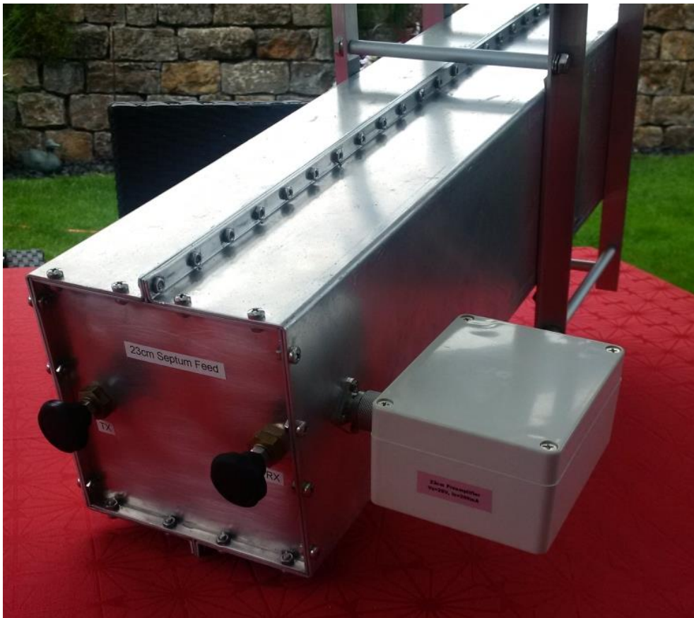
23cm EME low noise amplifier attached to RX port of Septum Feed
