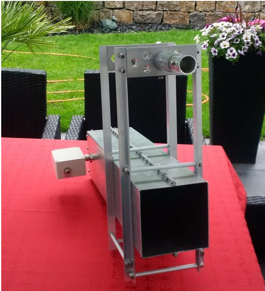
The Septum Feed needs a fare to make its beamwidth narrower to match my dish
