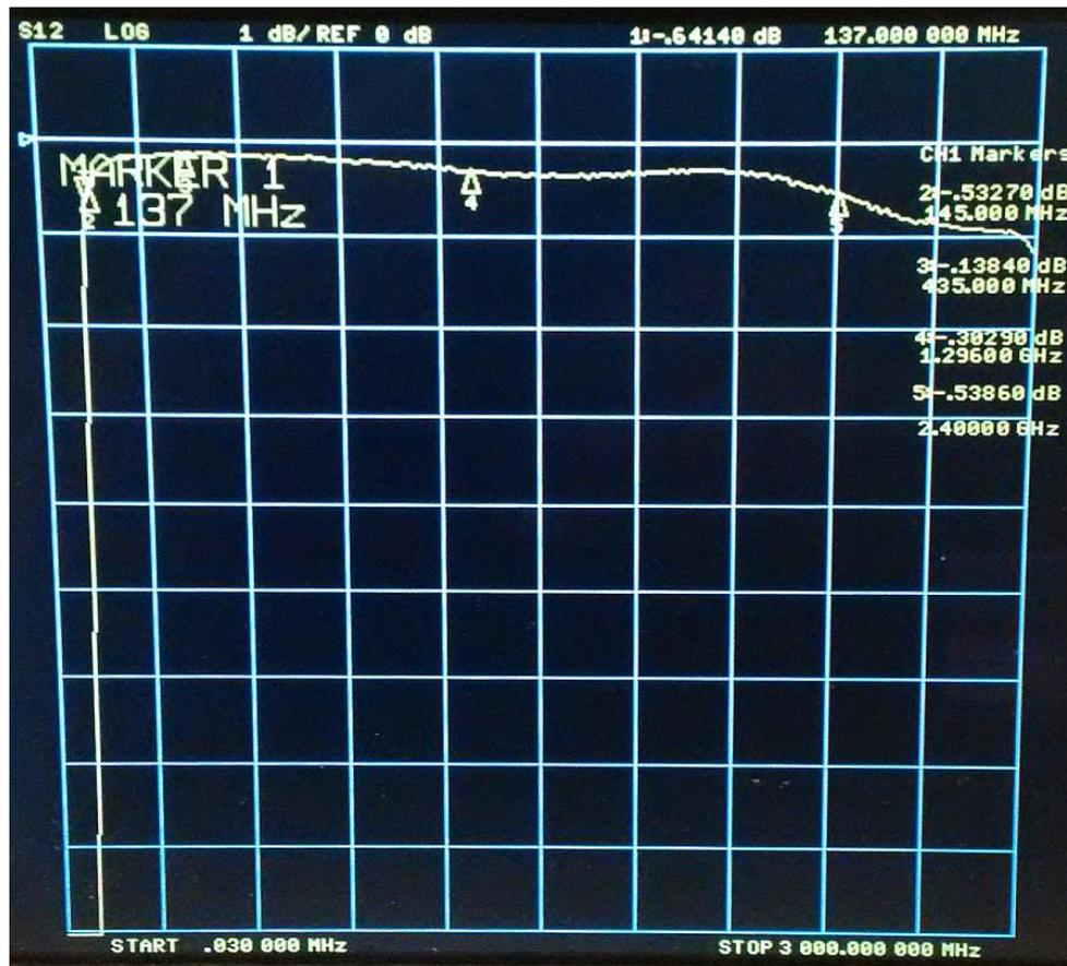
As the filter is symmetrical S21 and S12 are almost identical.
