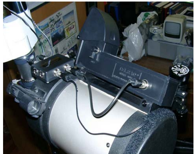
Top view of N5 with telrad finder, power distribution unit and corrector heater strip attached
