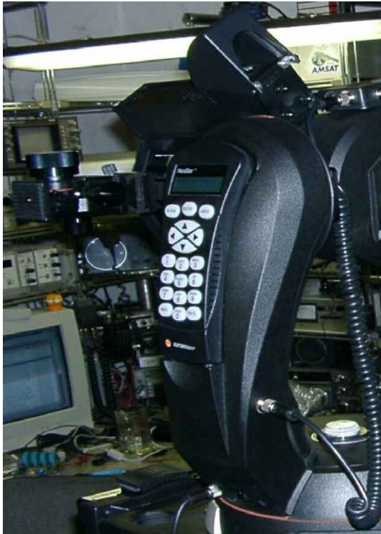
Side view of N5 with spiral cable from fork arm to power distribution unit on top of OTA
