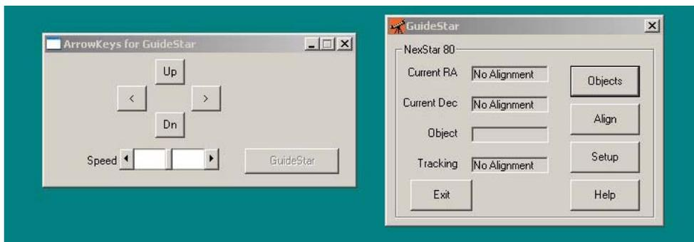
Of course you have to configure the „GuideStar“ software when you use it first time. Simply go through the setup menu and enter your location, time zone incl. daylight savings status, comm port number of the PC and your telescope model.
