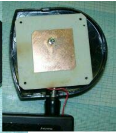
Patch antenna (on it's rear is the power amplifier PCB)
