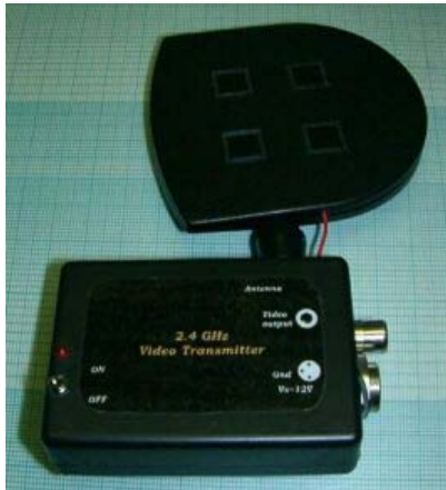
The complete video transmitter incl. antenna.
