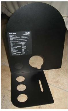
When I adapted my PST<sup>TM</sup> solar scope to my Celestron NexStar<sup>TM</sup> N5i mount using Ray's brackets I had to recognize that the Solar-Mate<sup>TM</sup> sun shield does not fit. I needed a design which was mirror-inverted and thus I decided to build one myself. This also gave me the opportunity to change the design slightly to optimize the relief to the NexStar<sup>TM</sup> N5i mount.
