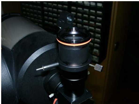
Fig. 3: Camera adapter with 35mm Baader-Eudiascopic Eyepiece attached to NexStar N5
