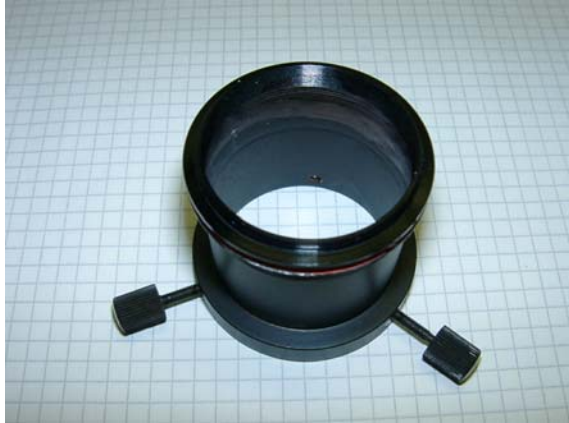
Fig. 1: Homebrew Adapter with 43mm thread – the eyepiece is fixed by the 2 thumbscrews
