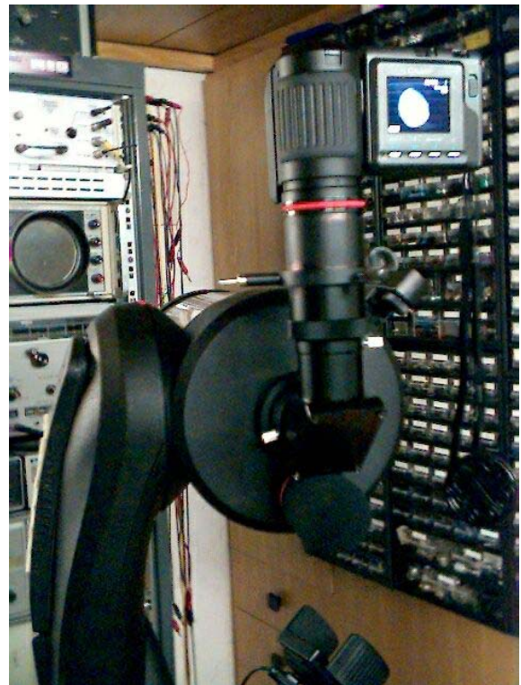
Fig. 4: Casio QV2800-UX digital camera attached to the N5 with the homebrew eyepiece projection adapter
