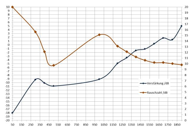
You can see that the gain (dark blue curve "Verstärkung" with the left scale) is negative at frequencies below 1600 MHz and the noise figure (brown curve "Rauschzahl" with the right scale) at 1600 MHz and above with 10dB quite high.
