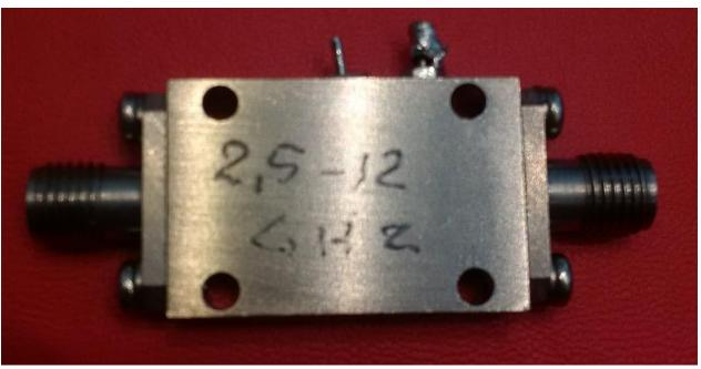
The handwritten frequency range is from the seller at the flea market. Apparently he verified that the amplifier works in the frequency range 2.5 to 12 GHz. No other data was available. The supply voltage of the amplifier is 5V and the supply current is 120mA.
