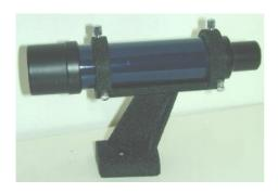
I found a low cost solution based on a simple 6x30mm finderscope. Such finderscopes can be found often on Ebay or Astromart for very little money – the optics is far from perfect but the bracket can be used to hold the laser instead of the finder. Thus we can make use of the possibility to adjust the laser relative to the main telescope.
