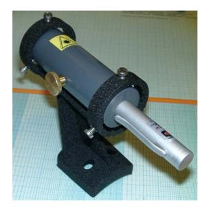
Now this assembly of laser pointer and cylinder around it can be inserted into the bracket and then attached to the telescope. The bracket features 2 rings each with 3 screws to allow an easy alignment of the laser pointer relative to the telescope.
