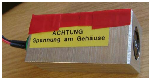
Laser module, the laser itself is supplied with -5V with the positive rail at the metal casing of the module, thus the casing is not grounded and some isolating tape is used.
