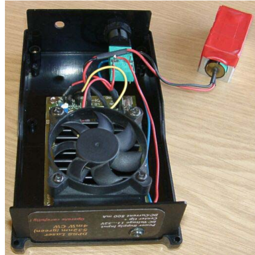
Rear view open, the fan cools the electronics, on the left at the free space behind the window (hole) is the place where the laser module will be inserted
