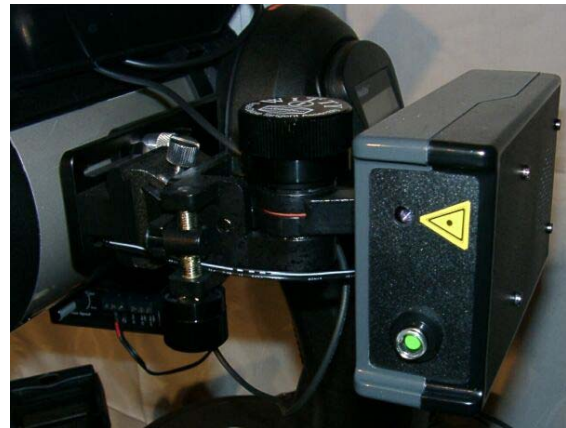
By means of a precise tangential adapter (called Witty One from Baader Planetarium) and the brackets from Ray Cooper (Ray's Brackets) I attached this laser to my N5. In the bottom of the case is a hole with a nut behind. Thus I can adjust the laser beam very precisely in all directions.
