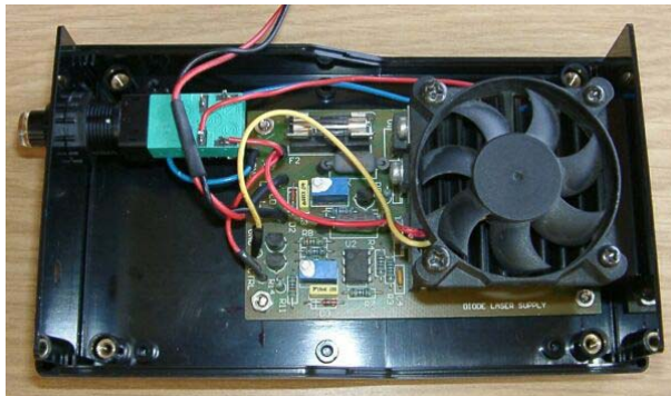
Side view open, the single PCB includes the power supply as well as the control circuit for the laser
