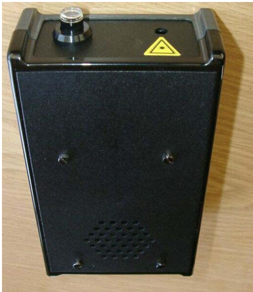
Front and top view, the holes on the top plate allow airflow into the case, the power button is at the front left, the laser output window at the front right
