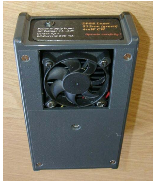
Rear and bottom view, the fan is needed to cool the electronics, the hole in the center includes a nut to attach the laser on a tripod or to the telescope
