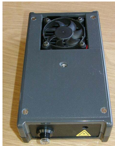
Front and bottom view, on the left the on/off button, on the right the window for the laser
