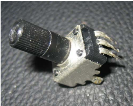
Defective potentiometer (1kOhm, linear)
