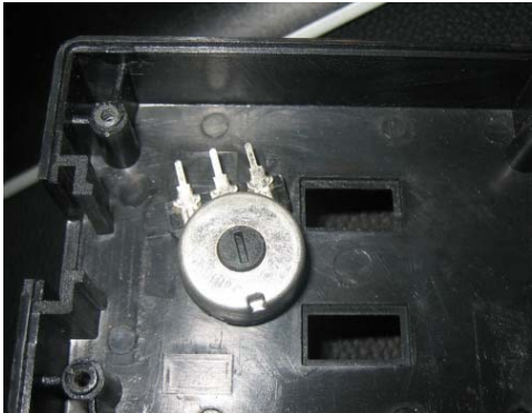
Replaced potentiometer (1kOhm, linear)
