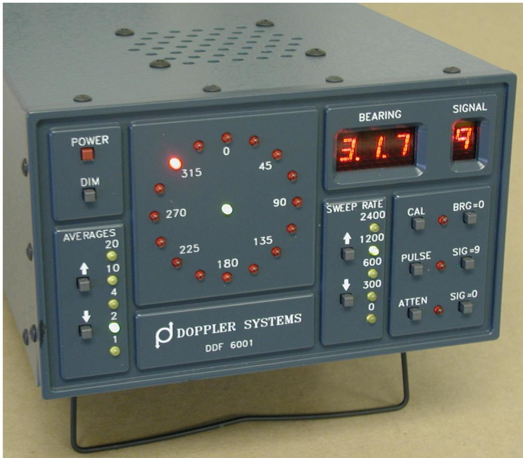
However one major difference is the interface to the RF summing unit and to the antennas. In this respect the DDF6000 and DDF6001 are **NOT** compatible.
