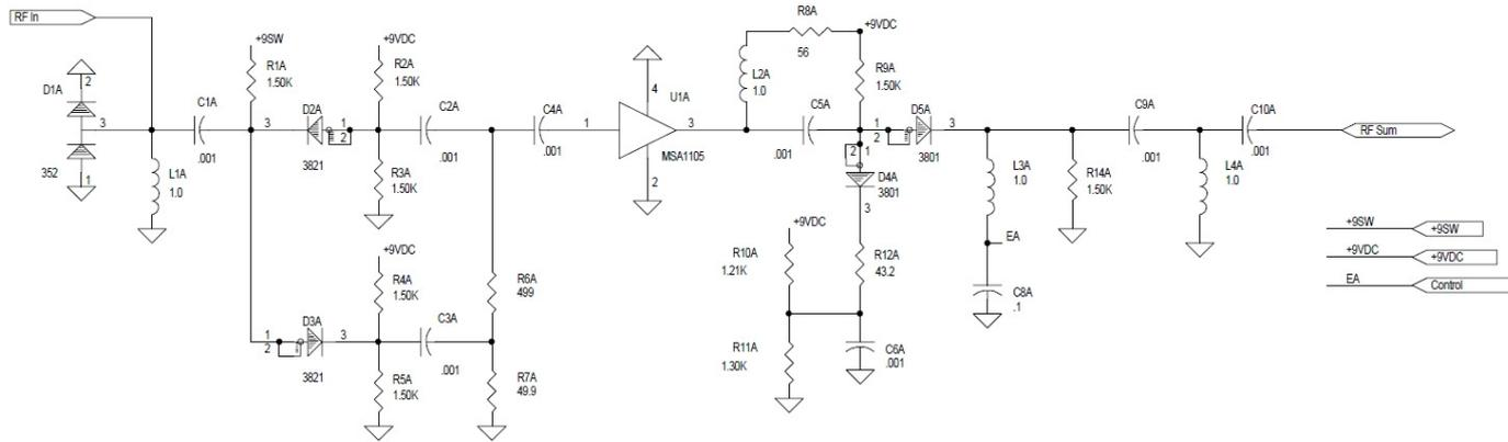
The electronics of each channel consists of a switchable 20 dB attenuator (comprised of D2A, D3A, R6A, R7A), a broad band amplifier (based on MSA-1105,  $G_p=13\text{dB}$ ,  $NF=3.6\text{dB}$ ), and an output switch (comprised of D4A, D5A, R12A) which either routes the amplified signal to the summing port or routes the signal to an integrated dummy load..
