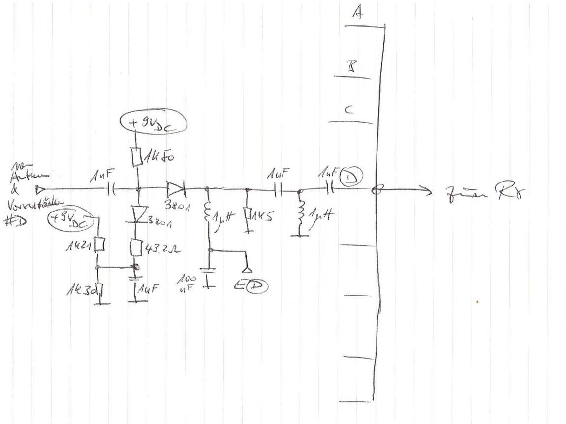
The PIN-Diodes “3801” are most likely of the type HMSP-3801 from Agilent.
