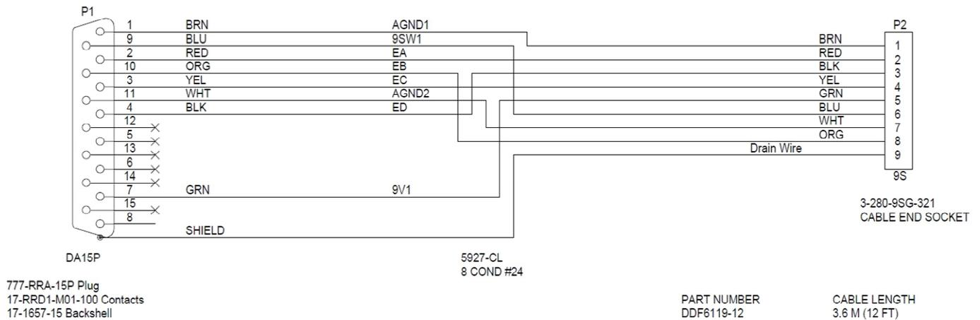
Here are descriptions for a 8 antenna setup. First the description of the necessary interconnections:
