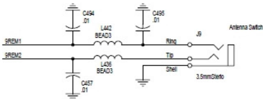
9REM1 and 9REM2 are output ports which are each internally connected via 350 Ohms to the +9V DC supply rail when enabled. They can thus drive directly small relays.
