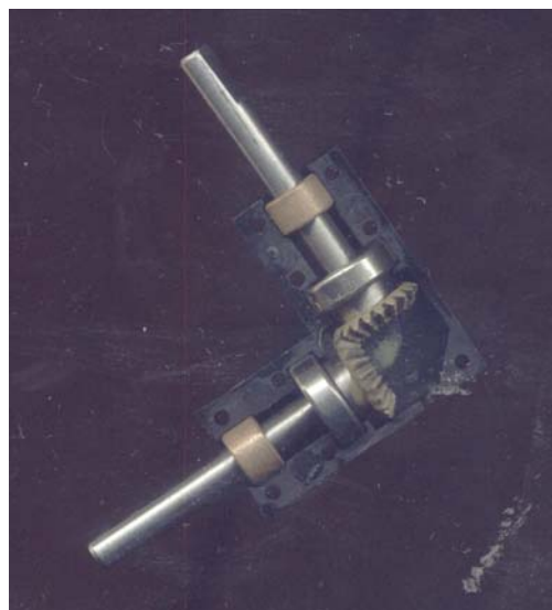
Gearbox opened to re-grease
