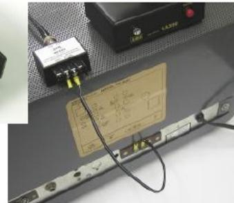
MC-600 is an optional interface between the 600  $\Omega$  antenna socket of your antique radio, and the 50  $\Omega$  input of the LA390 (or LA380) loop antenna. Supplied with a 30cm lead terminated with solderless terminals.
