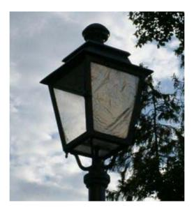
I just took a sheet of aluminium foil, opened the street lamp and shaded the window pane which is heading in the direction of my premise / observing location. The light which is no more disturbing me is not lost but reflected to the street opposite to my garden. I guess this is the least expensive and most effective filter you can imagine ;-)
