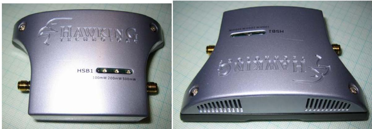
The device is supplied with a AC-DC power supply. The power supply provides 12V 1.5A to the Booster. I measured an averaged current consumption of 80mA in receive/standby mode and 200 mA in active mode (during a file transfer in 802.11g mode). Please note that WLAN is a TDD/TDMA system which means it uses
