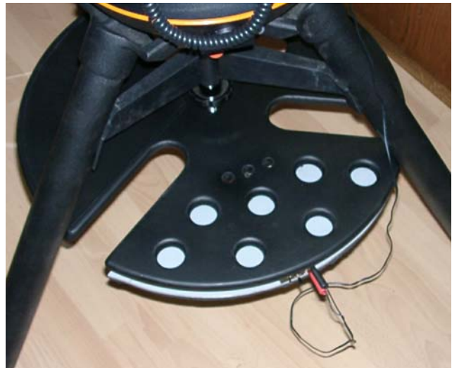
Accessory tray assembled as an additional spreader to stabilize the tripod
