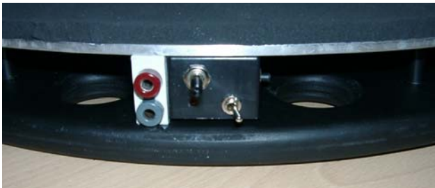
Power supply plugs and switches for red light and heater
