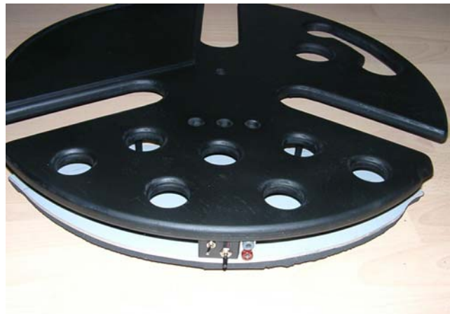
Side view of the tray with 12V DC power supply plugs and switches for heater and red light (between the wooden accessory tray and the metal heater plate below)
