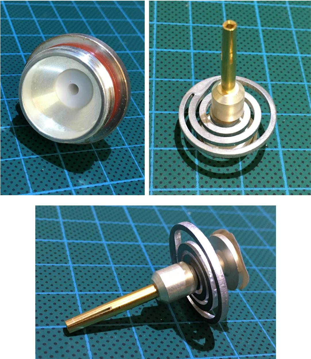
Thus, we can see that the lightning protector is a simple but very nice made high pass filter, consisting of an inductor to ground and a series capacitor. Here is a sketch of the simple schematic:
