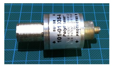
On the left side you see the N-Jack which is the unprotected side and should for instance be connected to the antenna, on the right side you can see the SMA-Jack which is protected and DC-decoupled from the antenna.
