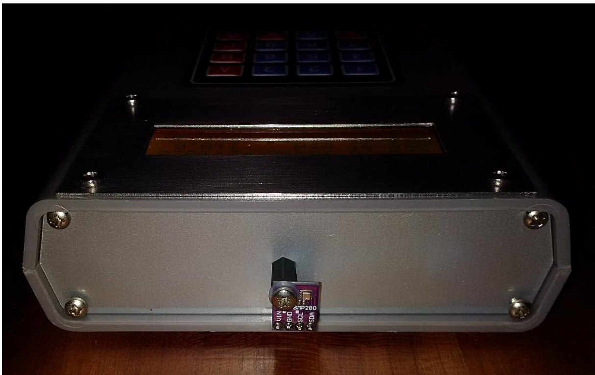
At the top end, outside of the Weatherbox, the small sensor board is attached
