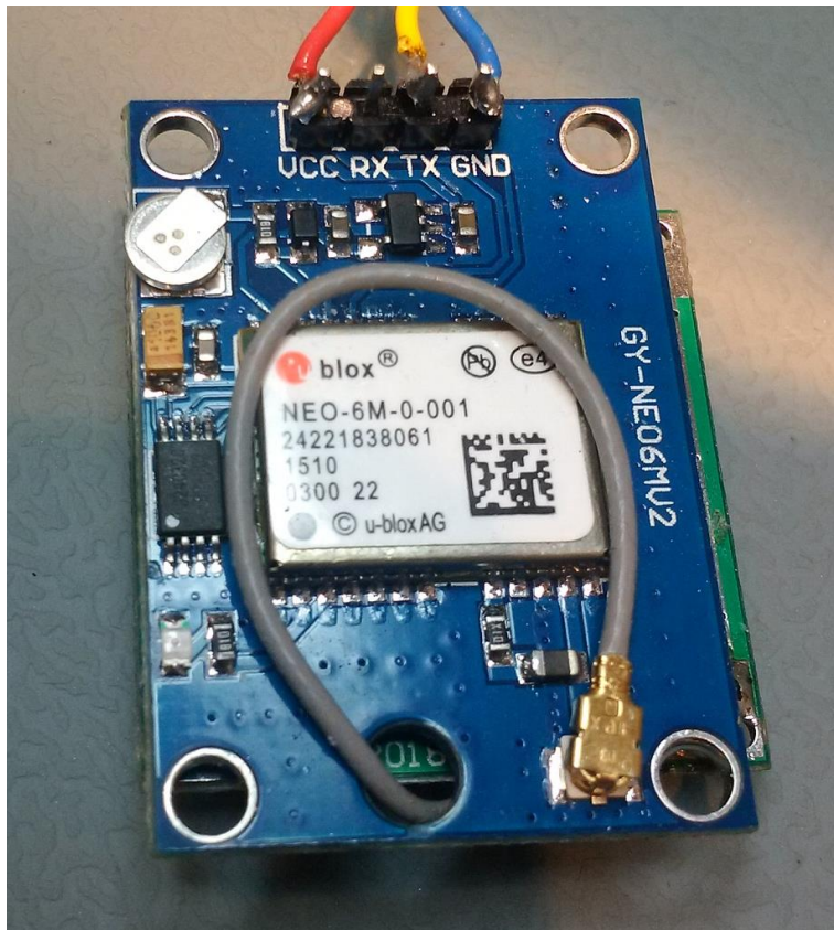
GPS board with ublox NEO-6M module (left) and sensor board (right)
