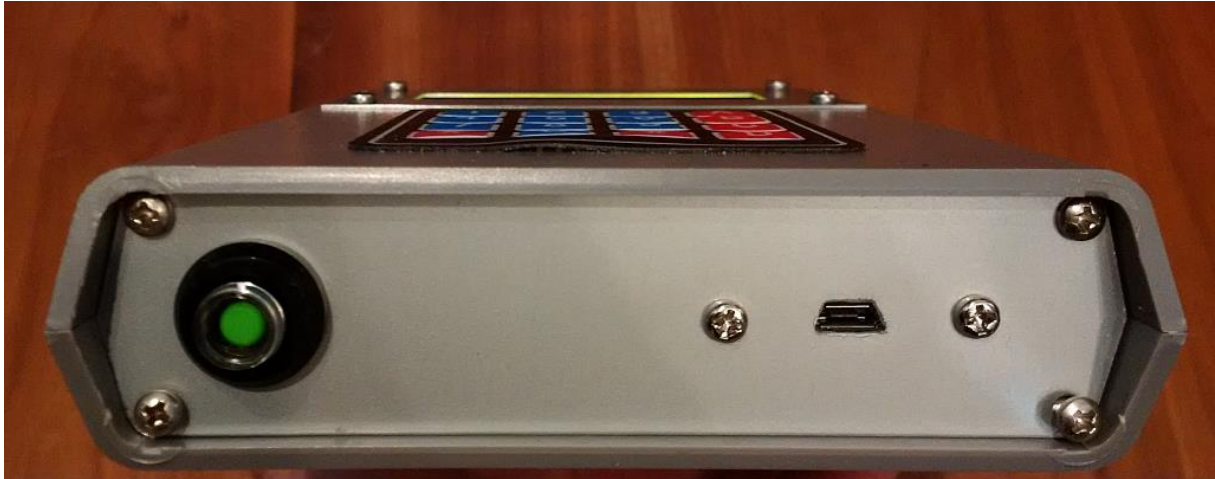
View of the lower end of the WeatherBox, on/off switch (left) and microUSB charging port (right)
