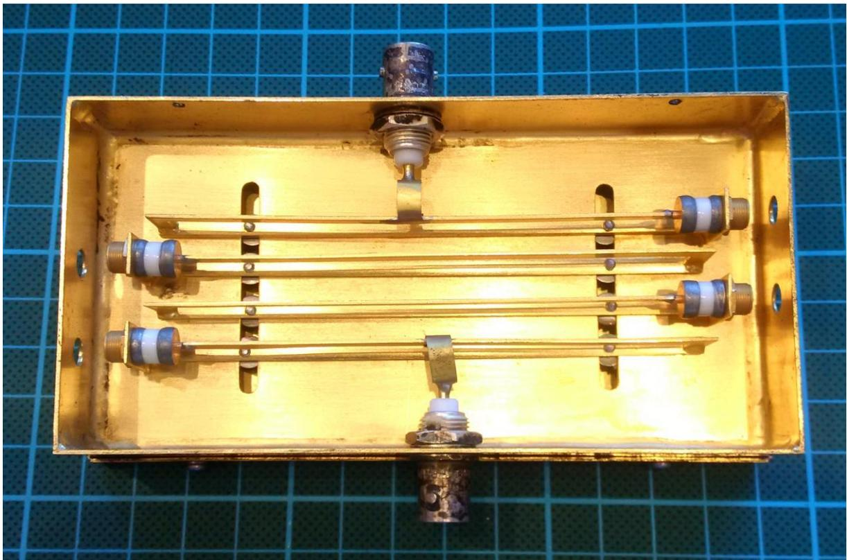
The filter consists of 4 parallel resonant tank circuits which can be tuned by high Q capacitors in center frequency. The coupling can be adjusted by moving the tank circuits laterally. I do not know why this filter is called fixed bandpass filter as it is highly flexible.
