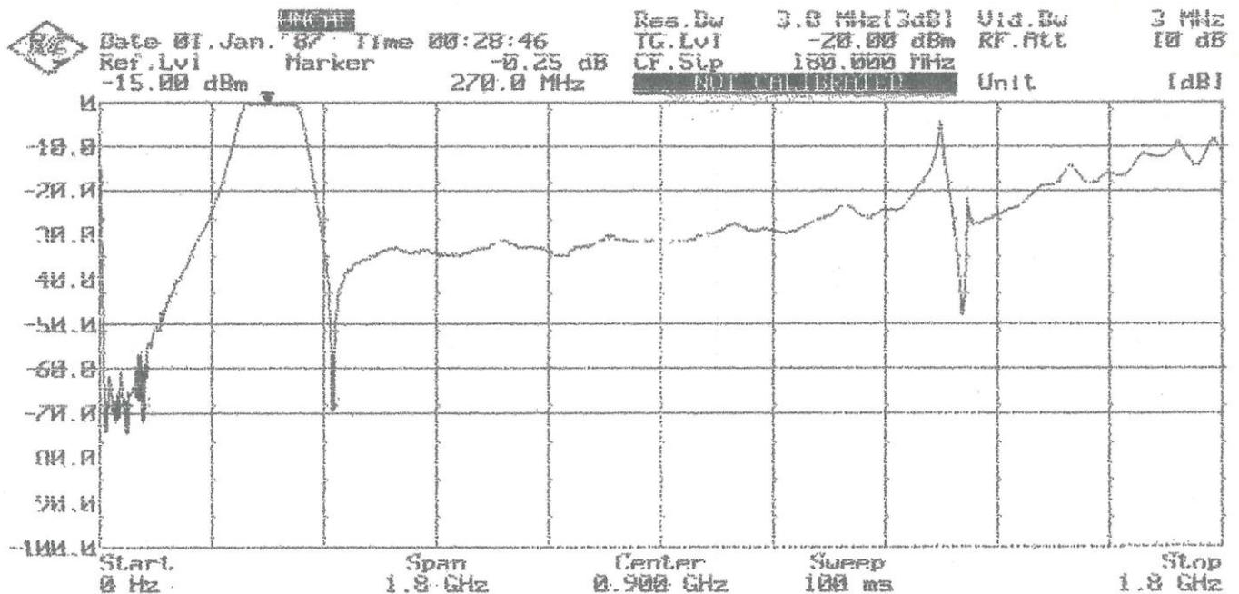
The filter response in the passband is quite flat. Below the passband the rejection is about 50dB in the 100 MHz broadcast radio band. Above the passband the rejection is only about 35 dB (30dB above 1 GHz). There is a spurious response in the range of 1350 MHz which is no problem in my application.
