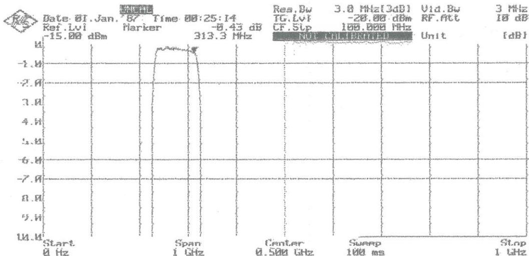
The upper bandwidth after retuning is still a bit high which was no problem in my application. The filter has now an insertion loss of better than 0.3dB between 240 and 300 MHz.
