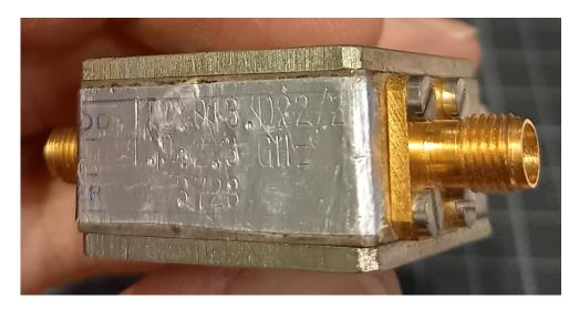
The isolator is housed in a solid metal case and female SMA connectors are used at the input and output ports.
