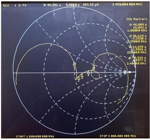
The measurements results of this isolator at 2.320GHz show that it is well suited to be used at this frequency.
