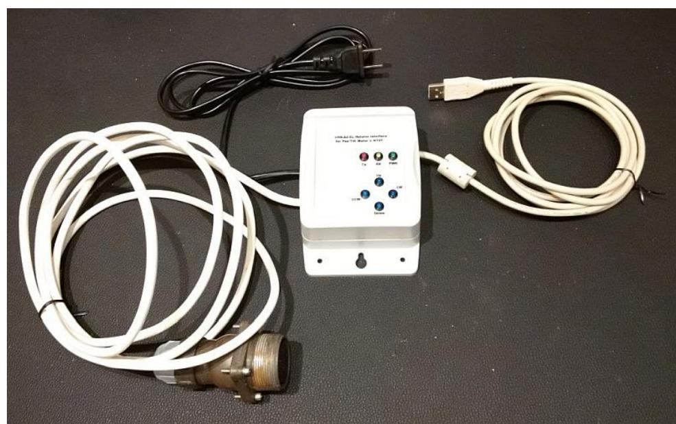
The controller is powered by the USB-port. The mains cable will supply the 110V for the rotator. The relays inside the controller switch the respective rotator ports for turning in CW/CCW respectively UP/DOWN directions.
