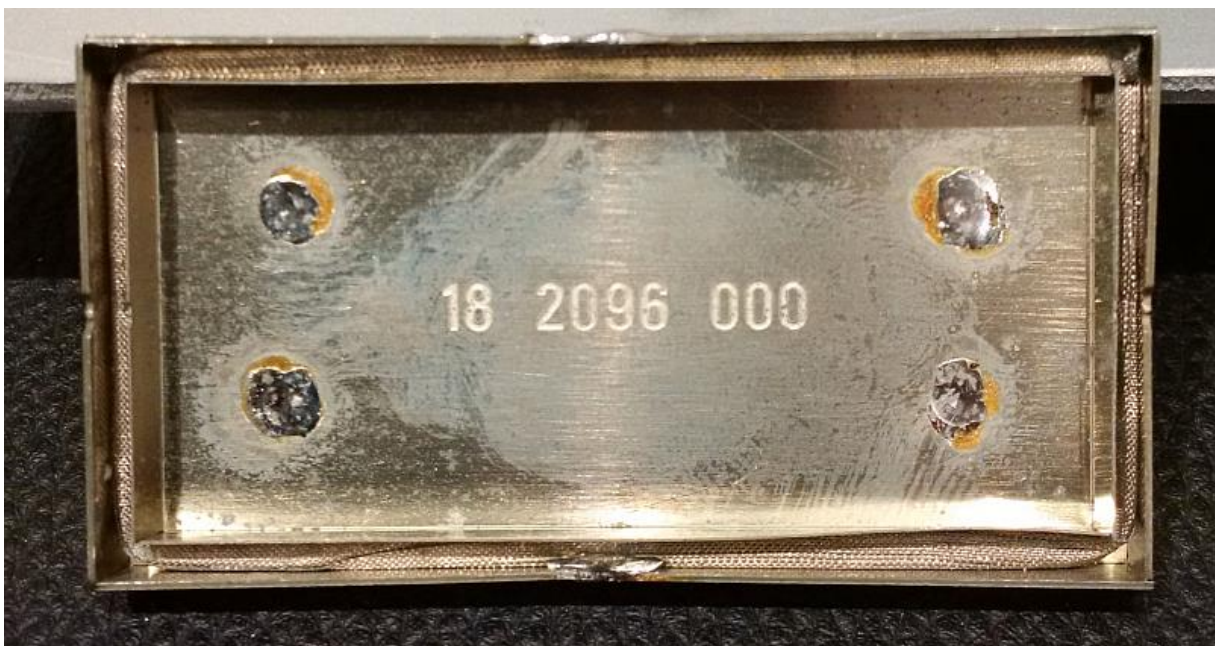
The tin-plated cabinet has an interesting lid. It is comprised of 2 lids which are soldered together and there is an embedded metal netting to guarantee a proper contact between the lid and the encasing.
