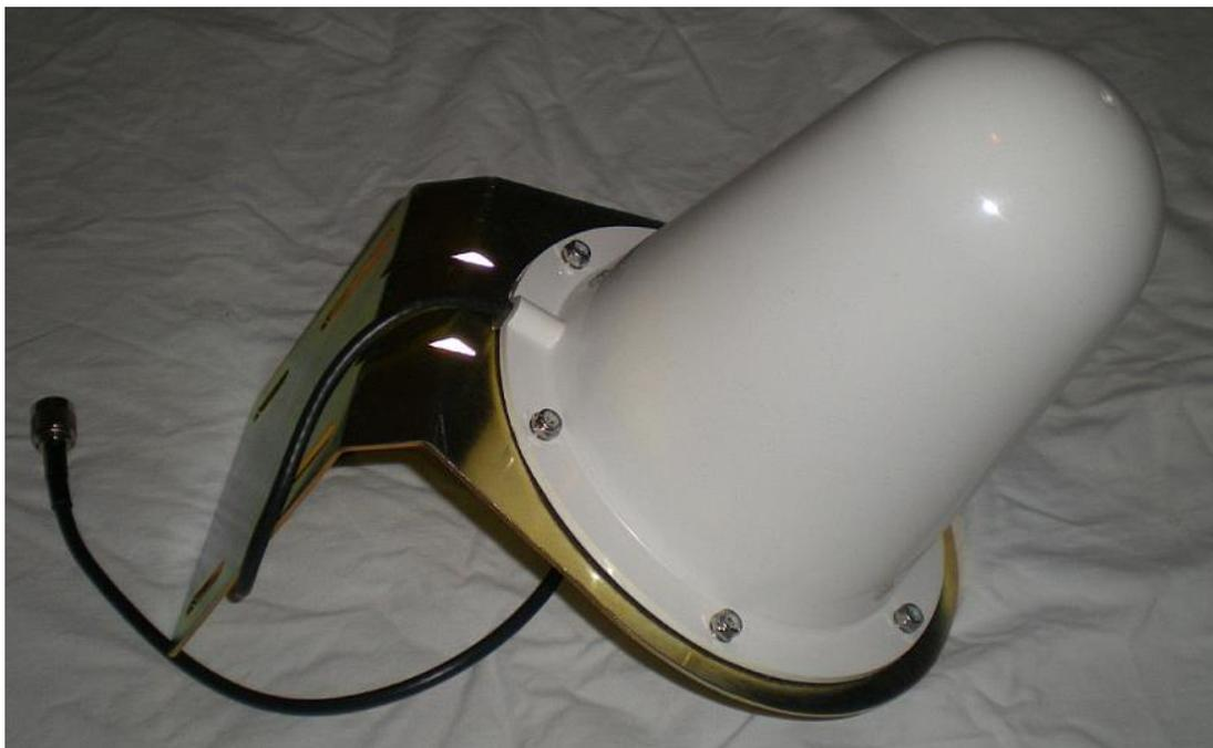
This antenna is housed in a plastic radome and has already a bracket attached to it. Inside the radome was a quarter wave ground plane antenna.
