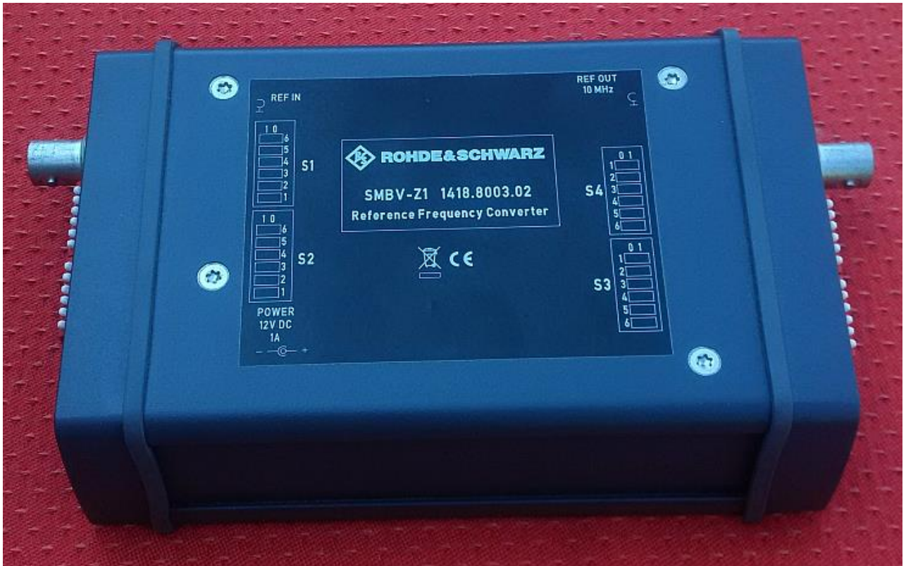
Input and output connectors are BNC type, on the left is the REF IN port, on the right is the 10 MHz REF OUT port
